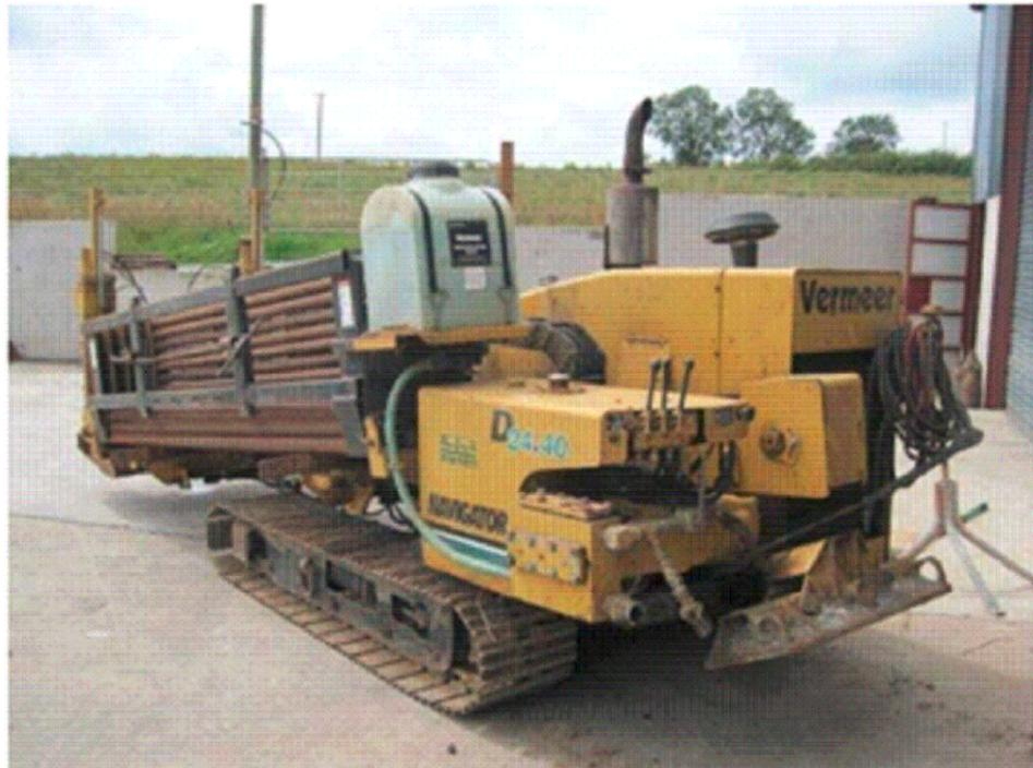
Image 1 : Directional Drilling Rig
